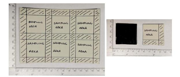
Figure 6. Image of whole gellifter marked for sampling, and front and back images of individual section of gellifter used to lift one fingerprint. Hatched areas represent border handling areas. Image: Authors own.
