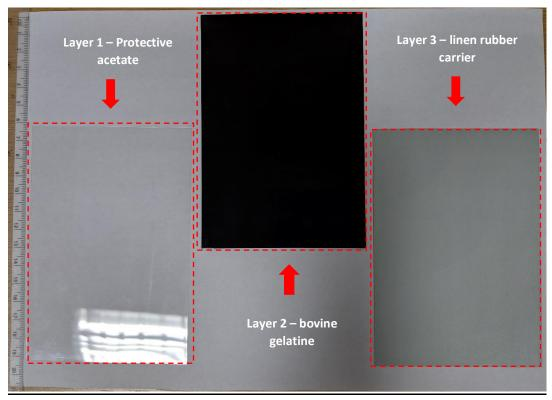
*Figure 2. Diagram of deconstructed gelatine lifter with individual layers outlined in red. Layer 1 protective acetate. Layer 2 bovine gelatine. Layer 3 linen rubber carrier layer, Image: Authors own.*
